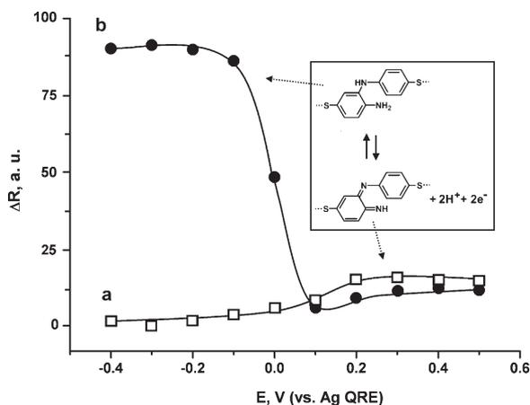
**Figure 3.** Effect of applied potential on the reflectance changes, at  $\theta = 63.6^\circ$ , of the Kemp's acid-imprinted composite of bisaniline-crosslinked Au NPs: (a) The imprinted composite in a pure 0.1 M HEPES buffer solution at pH 7.2 and (b) The imprinted composite in a 0.1 M HEPES buffer solution at pH 7.2 that included 300 fM RDX. Inset: the redox states of the bisaniline bridges.
