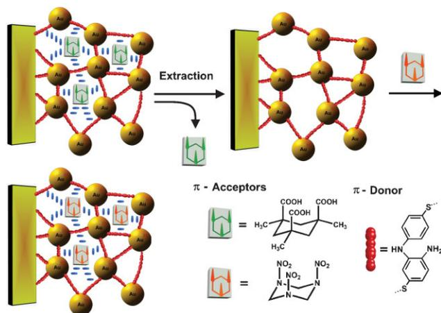
**Scheme 1.** Imprinting of Kemp's acid molecular recognition sites into the composite of bisaniline-crosslinked Au NPs associated with a Au electrode, for RDX analysis.
