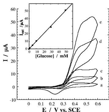
**Fig. 1** Cyclic voltammograms of the Au electrode modified with the PQQ-functionalized polyaniline/polyacrylic acid film and the reconstituted GDH in the presence of various concentrations of glucose: (a) 0 mM, (b) 5 mM, (c) 10 mM, (d) 20 mM, (e) 50 mM. The data were recorded in 0.1 M phosphate buffer, pH 7.0 under air, potential scan rate 5 mV s<sup>-1</sup>. Inset shows the calibration plot of the electrocatalytic current vs. glucose concentration.
