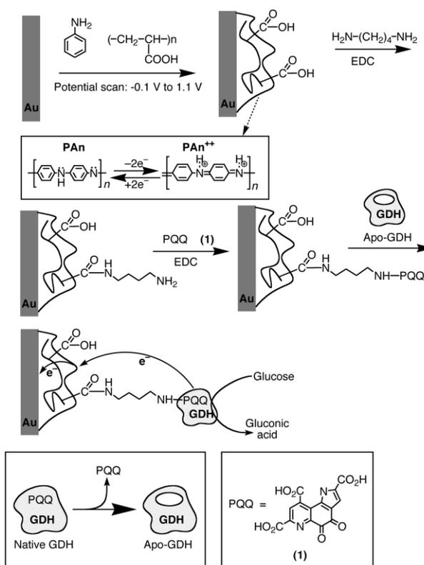
**Scheme 1** Reconstitution of glucose dehydrogenase (GDH) on the PQQ-functionalized polyaniline/polyacrylic acid film associated with an Au electrode.
